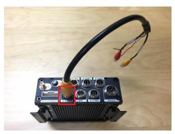
3. XDR Rear – Connect **EX4-NPIG** to **AV-OUT** port on XDR for video out connection to monitor. May need BNC to RCA converter
