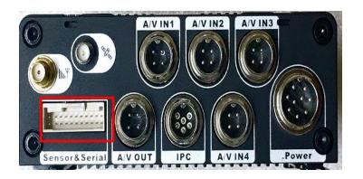
2. Connect EX4-ALC (Sold Separately) to Sensor/Serial Port. Connect EX4-PGM to EX4-ALC
