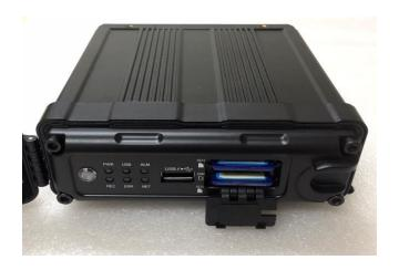
1. XDR Front Panel – SD Card Slots, USB Port and System LED
