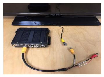
4. XDR Rear – Connect EX4-NPIG to RCA video connection to monitor to monitor
